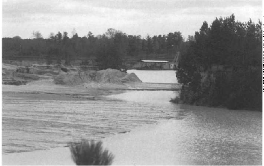
Dredged sand is placed along the shoreline of the Amite River, Louisiana, for processing.
